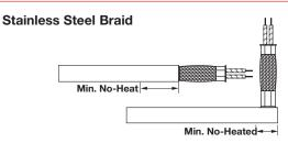
A stainless steel braid is designed to protect leads from abrasion against sharp edges. It is the most flexible of Watlow's protective lead arrangements.
