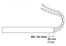
Swaged-in flexible leads, with silicone-fiberglass insulation, are recommended for applications in which the leads must be bent at the exit point from the heater. Unless longer length is specified, 250 mm (10 in.) leads are supplied.
