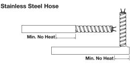
Stainless steel hose provides the best protection against abrasion from sharp edges or abrasive equipment. It also offers ease of handling and wiring in abrasive environments. When the leads exit at a right angle to the heater, the hose is silver soldered to the sheath. Unless otherwise specified, leads are 250 mm (10 in.) long and the hose is 200 mm (8 in.) long. To order, specify **stainless steel hose**, lead length and no-heat section.
