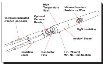
\* First 3 in. (76 mm) at lead end must be kept below 1000°F (538°C)
