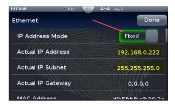
8. The computer and F4T are ready for communications. Use either Composer software or Modbus TCP software of your choice for communications via Ethernet.
