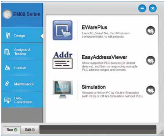
Utility Manager uploads and downloads projects to and from the Silver Series EM OIT, opens compiled projects in simulation and launches the other EZwarePlus programs.
