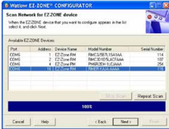
Detects EZ-ZONE devices connected to the computer's communications ports.
