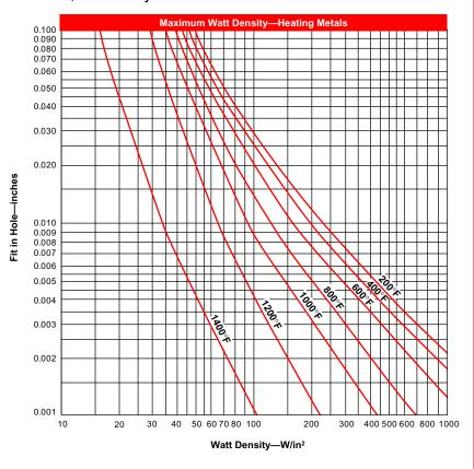
Correction Factors: Also note, this graph depicts cartridge heaters used in steel parts. Therefore, for either stainless steel or aluminum and brass, refer to applicable correction factors:
