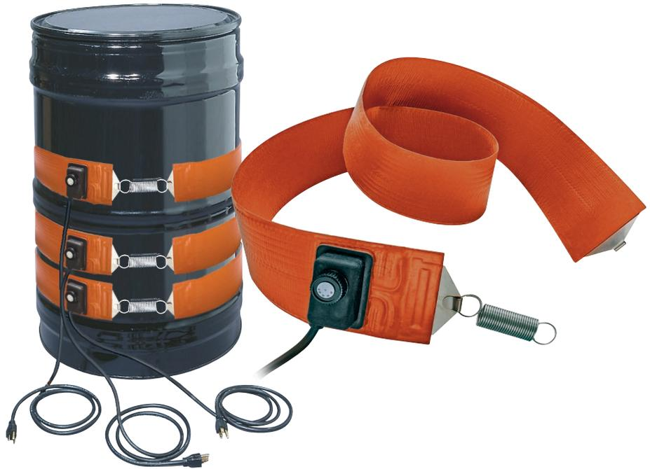
Chromalox PHD heavy-duty fiberglass woven drum heaters are constructed of fiberglass-insulated resistance wire woven into a mesh blanket and then encased in layers of silicone rubber. Like Chromalox SLDH silicone-rubber-insulated drum heaters, PHD fiberglass
