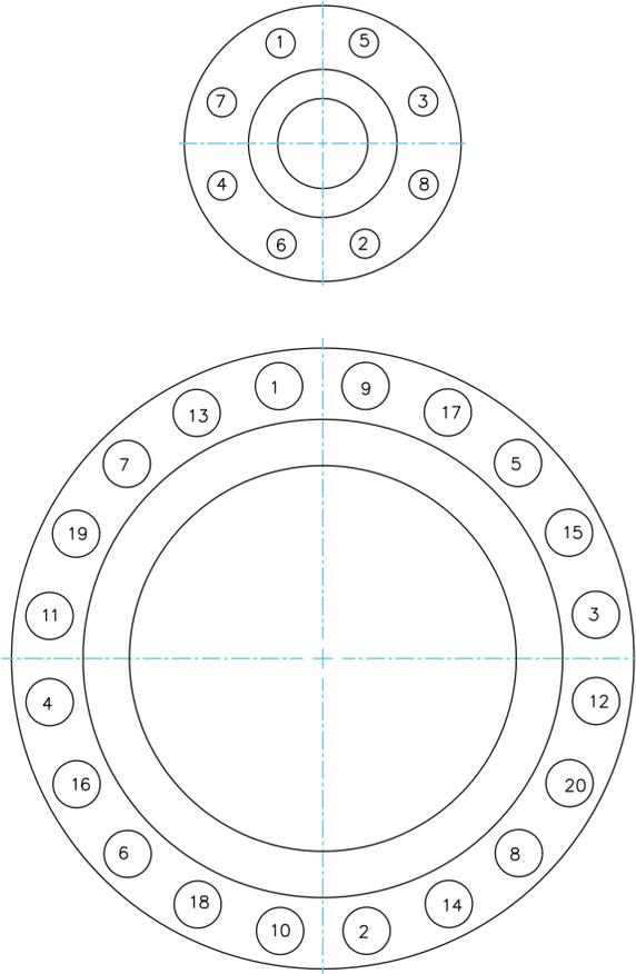
A tightening sequence similar to that shown in Figure 2 is recommended for use until any angular misalignment is taken up. When flange faces are parallel the tightening sequence shown in Figure 1 shall be used.
