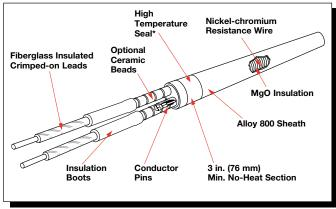
\* First 2 in. (51 mm) at lead end must be kept below 1000°F (538°C).
