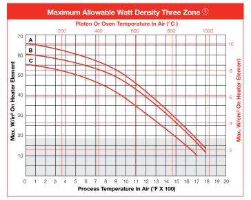
A = 6 cell, 0.935 in. diameter, 240VAC, 3-phase B = 6 cell, 0.685 in. diameter, 240VAC, 3-phase
