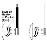
Flexible Stranded MGT Insulated Nickel Lead Wire (450°C Rated)
