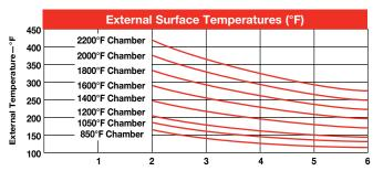
Total Wall Thickness-inches (Includes Standard 2 in. Heater Thickness)
