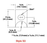
Tabs and rings are used to hold the heater in place and keep it from creeping. Available in carbon steel, 304 and 316 SS.
