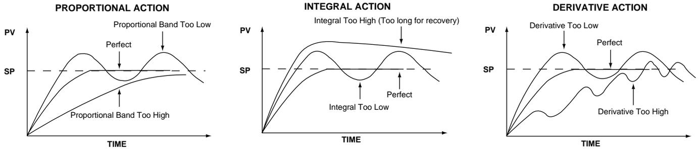
Fig. 5.2 Effects of PID Adjustment of Process Response
