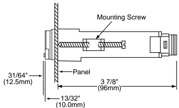
*Controls are supplied with mounting clamp and mounting screws. Release the mounting clamp by depressing the ends of the clamp together. The mounting screws are to be used in applications that require NEMA 4X rating.*
