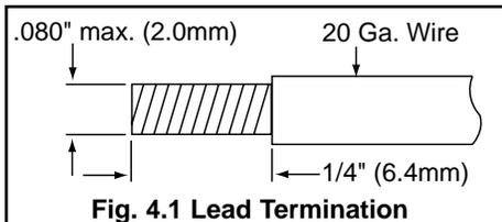
**Fig. 4.1 Lead Termination**
