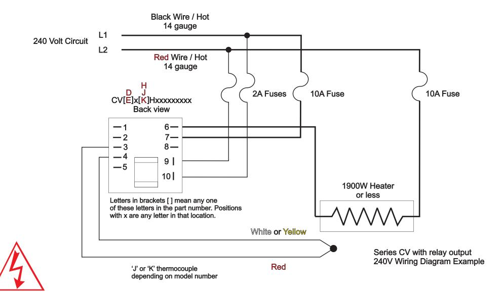
Warning: Use National Electrical Code (NEC) or other country-specific standard wiring and safety practices when wiring and connecting this controller to a power source. Failure to do so may result in damage to equipment and property, and/or injury or loss of life.
