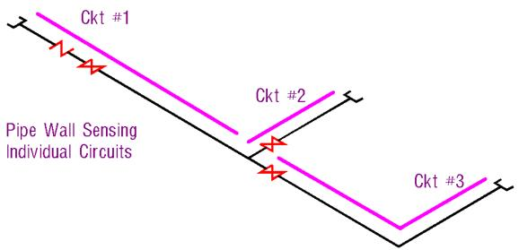
Illustration 30: Flow Path/Circuit Analysis – Pipe Wall Sensing
