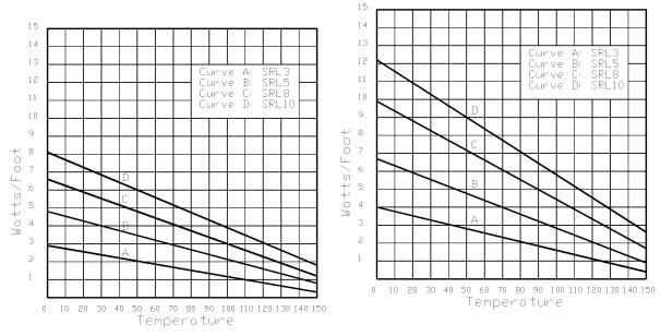
\*Graph 5 and Graph 6 extrapolated from Chromalox® Design Guide PJ-304-1 to illustrate difference in cable output.
