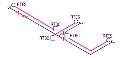
The RTBC enclosures are positioned together to centralize the power wiring and conduit. Most contractors and facility maintenance personnel prefer this method unless specific requirements dictate that controllers be located at a particular point.
