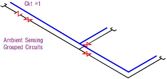
Illustration 32: Flow Path/Circuit Analysis – Ambient Sensing
