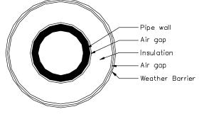
Equation 1.4 is based on the heat loss of an *entire* flat area where the inside area of the insulation wall is the same as the outside area. To simplify heat loss calculations pipe heat loss is based on the heat loss per linear foot rather than the entire area of any given length. Also, for pipe insulation, the outer area of insulation is greater than the inner area due to wrapping insulation around the cylindrical
