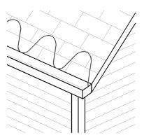
Snow melting cable is not intended to completely melt the snow and ice from a rooftop. Rather, it is intended to
