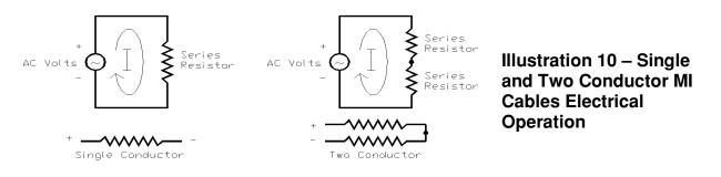
To assemble an MI cable, the exact length and construction style must be known since it affects whether the unit can be manufactured. Because of welding and testing procedures involved in MI cable assembly, MI cables are always factory assembled. Consequently, all construction information must be known in advance of manufacturing. Field modifications are extremely difficult because changes in length or voltage affect the overall cable output wattage.
