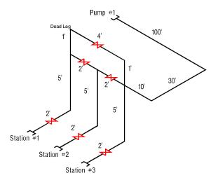
How many flow path circuits are in Illustration 31, including common pipes?
