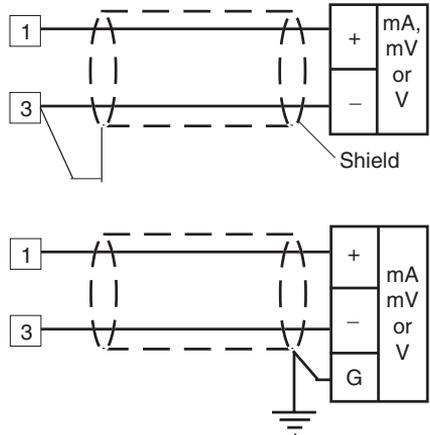
Fig. 6 mA, mV AND V INPUTS WIRING
