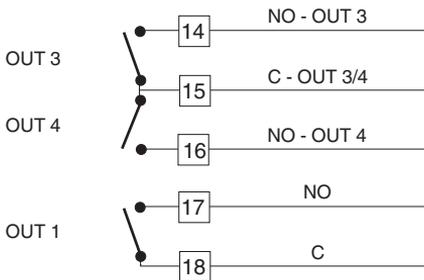
Fig. 9 RELAY OUTPUTS WIRING
