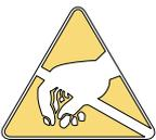
**It is not necessary to remove the control chassis from the housing for installation. If the control chassis is removed from the housing, you must follow industry standard practice for control and protection against Electro-Static Discharge (ESD). Failure to exercise good ESD practices may cause damage to the control.**
