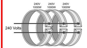
**SERIES WIRING:** ILLUSTRATION SHOWS 240V BANDS WIRED TO
