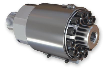
**MDi's Dual Stage Filter Device** eliminates gate obstructions caused by contaminants that can be inadvertently introduced into the molding material. Mounted between the extruder barrel and the molding machine nozzle, our unique design works to protect critical mold components by using two separate melt stages.
