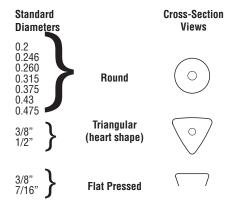
Round Cross Section — Highly adaptable where elements must be bent — particularly if bending is performed in the field.
