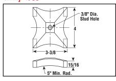
**Clamp 5970** — Use to clamp three strip heaters on 2" centers using 5/16" studs at 5" intervals (PCN 263652).
