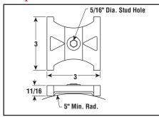
**Clamp 6933** — Use to clamp two strip heaters on 3" centers using 3/8" studs at 5" intervals (PCN 263644).
