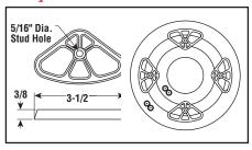
**Clamp 5971** — Use to clamp two strip heaters on 2" centers using 5/16" studs spaced 5" apart (PCN 263636).
