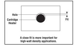
**Determining Watt Density** — Watt density refers to the heat flow rate or surface loading. It is the number of watts per square inch of heated surface area. For calculation purposes, CIR stock cartridge heaters have 1/4" unheated length at each end. Thus, for a 1/2 x 12" heater rated 1,000 watts, the watt density calculation would be as follows:
